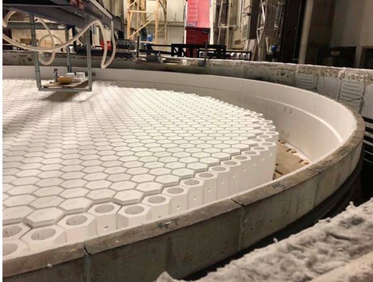
Figure 6. Nearly completed mold for casting GMT Segment 6.
