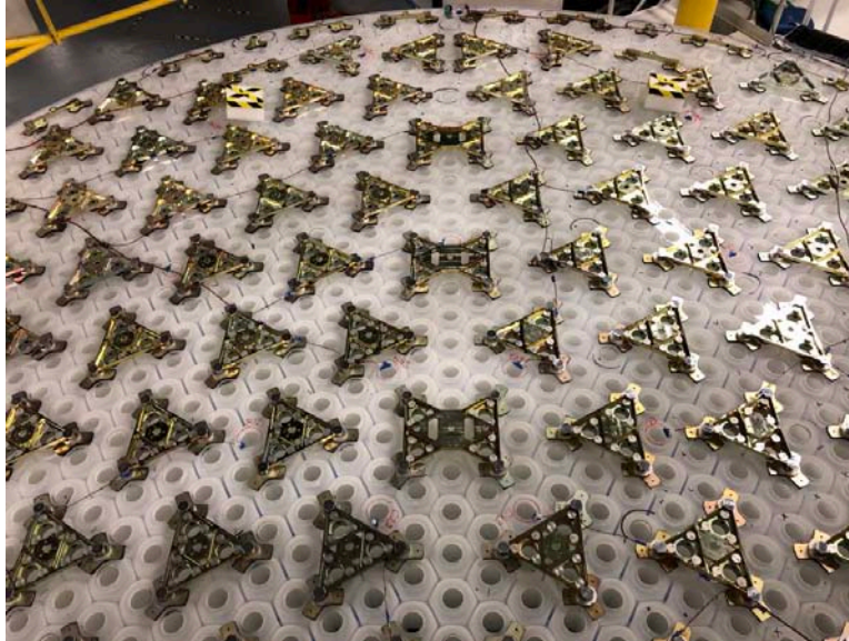
Figure 4. Rear surface of Segment 5 showing some of the 165 loadspreaders. In the telescope, each loadspreader is the interface to a 3-axis (axial + 2 lateral) pneumatic actuator.
