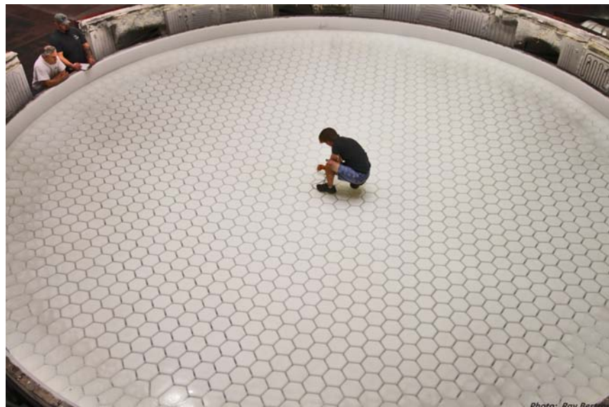
Figure 3. Measurement of the thickness of the facesheet after the spin-casting of GMT Segment 5. Photo by Ray Bertram, University of Arizona.
