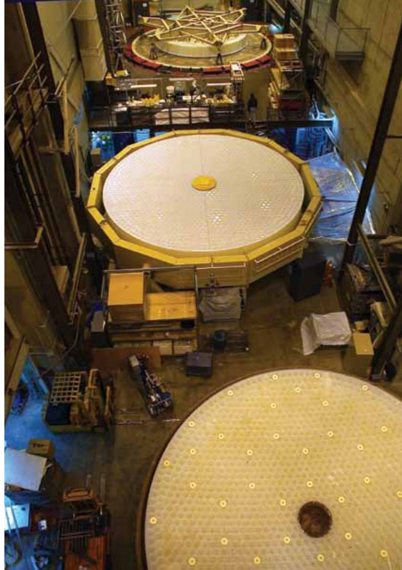
The two 8.4-m primary mirrors for LBT were spun cast at the Steward Observatory Mirror Lab in 1997 and 2000. They are shown here in the casting lab in January 2003 when rough abrasive grinding had been completed. In the background is a 6.5-m mirror for another project. Note the senior staff technician, Damon Jackson, on the upper right at the top of the stairs.
