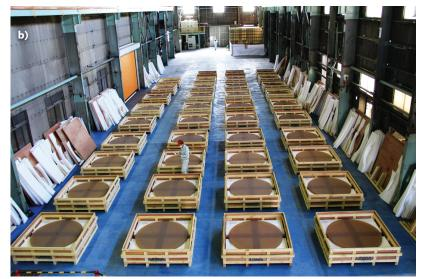
CLEARCERAM-Z HS boules produced at Ohara's factory in Japan (a) will be further processed to become the M1 primary mirror segment blanks that, when placed in a closely fitting hexagonal array, will form the TMT's primary. Some of the more than 100 mirror blanks already produced by Ohara undergo an inspection (b). *(Courtesy of Ohara Corp.)*
